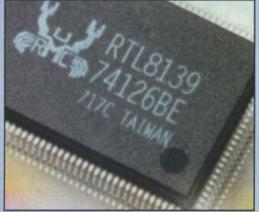
Realtek Semiconductor integrates Fast Ethernet onto a single chip.
